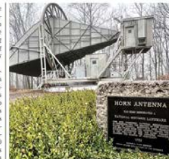
Scientists used the 30-foot aluminum antenna atop Crawford Hill in Holmdel — one of the highest points in Monmouth County — to prove the Big Bang, a theory of the creation of the universe.
